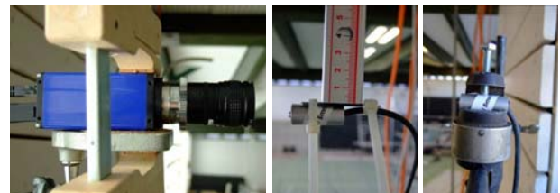
Figure 2: Preliminary tests, system components: Camera (left), movable LED-target as measuring point (center) and LED-target as reference point (right)
